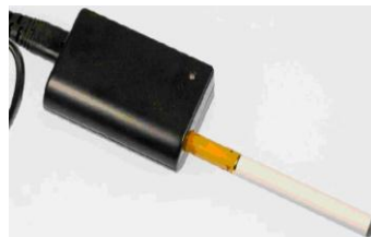
Image of an electronic cigarette inserted into a charger
